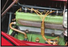
mitted through a cone clutch to the rear transaxle. The transmission had three forward gears, and one reverse. A double drop frame was used to keep the car closer to the ground. The suspension for the car consisted of semi-elliptic springs on the front, and full elliptic springs on the rear. Brakes were provided on the rear only. Thirty four inch wood spoke wheels mounted with thirty four inch x three and a half inch tires, was standard on these automobiles.
